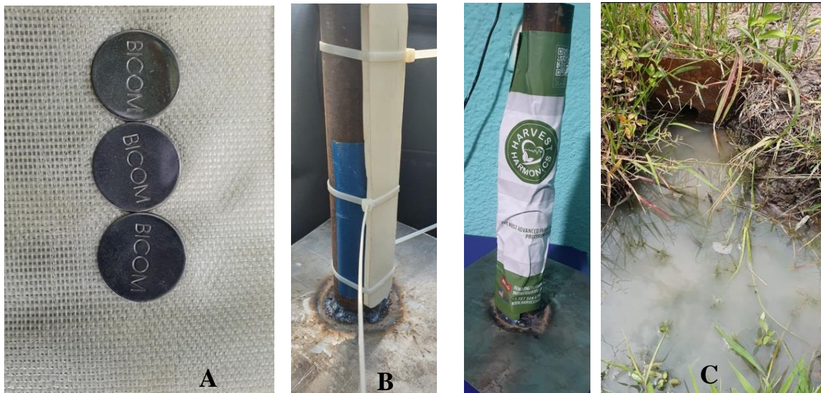
Figure 1: Crop Booster device (A= micro-transmitter; B= irrigation tube with micro-transmitter; C= irrigation device installed)
